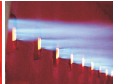
Rekumat M200 burner firing into an open combustion chamber in Flame mode
